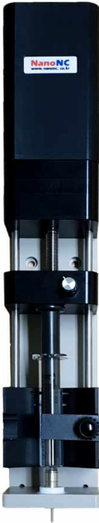
10cc syringe setup on pump *no cylindrical metal guide
