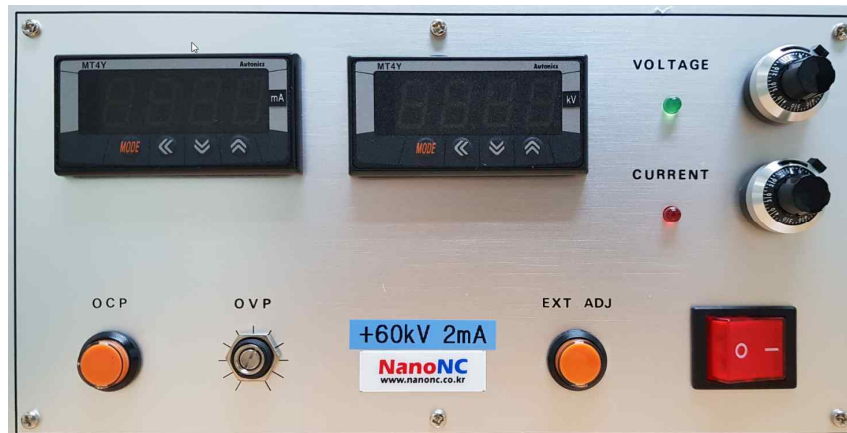
(Front Part of HV Power Supply)
