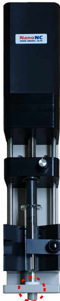
The attachment of cylindrical metal guide : stable electrospinning at nozzle tip
