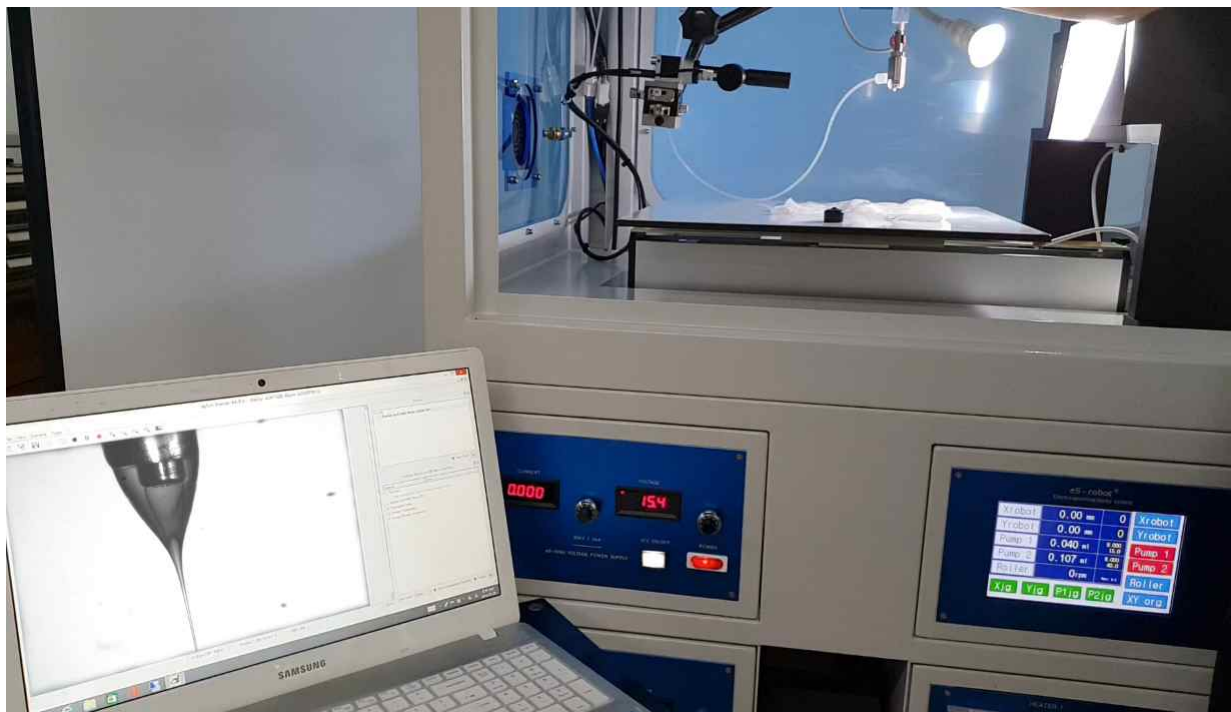
(Setup of Vision Camera for Electrospinning with Coaxial Nozzle)
