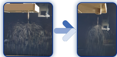
formation of a stable taylor cone on nozzle tip in applying a higher voltage
